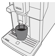
**Note:** to prepare two cups of espresso or long espresso, press the button of the preferred beverage twice. The machine performs two consecutive grinding cycles automatically.
