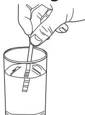
Use the supplied stripe for measuring the water hardness.
